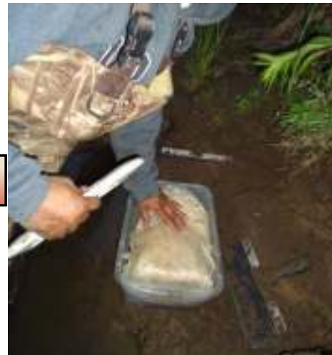
The soil block was covered with plastic sheet and stored in a box.
