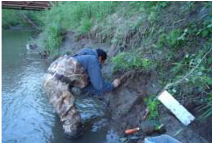
A Soil block (35 cm x 20 cm x 15 cm) was cut from the bank.
