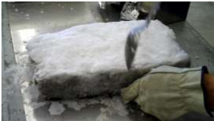
The soil block was wrapped with cheese cloth and waxed.
